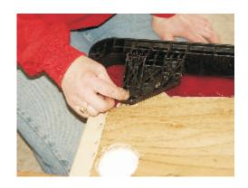
1.) Remove side handles and mounting hardware from stock seat base.
