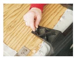
2.) Install handles and hinge tabs on base of Suite Seat. \*IMPORTANT\* Hand start all bolts to prevent damage to t-nuts. Seat base can now be installed on cart.
